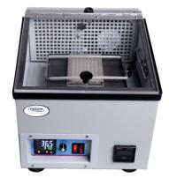
**MICROPLATE SHAKER** provides regulated shaking for two micro plates. With a speed range of 200 to 1500 rpm, it can be adjusted to suit gentle shaking to ensure that the well contents are not ejected or more vigorous agitation for effective aeration across the small surface area of each of the wells. They are suitable for mixing, incubation and cultivation of biological and chemical components.
