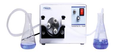
**PERISTALTIC PUMPS** work on principle of "Positive transportation of fluids by cyclic contraction and expansion of Flexible tubes:. A Silicon Rubber tube supported by a semicircular stage and is squeezed by three rollers cyclically for creating suction head and pushing forward the liquid or gas. There are many advantages in this method of fluid handling.
