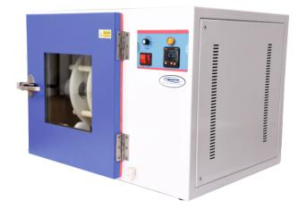
**HYBRIDIZATION OVENS** are used in research labs, molecular biology labs, and other labs to identify RNA, DNA, and proteins. They are used for nucleic acid and protein hybridizations, and are especially useful for Northern, Southern, and Western blots.
