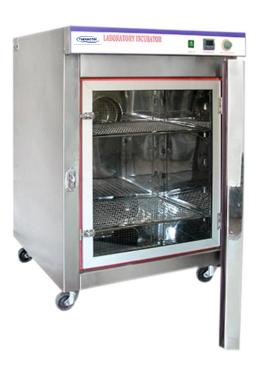
**BACTERIOLOGICAL INCUBATORS** are designed to serve a wide span of requirements, most useful for General Incubation, Excellent for usage in Microbiological Labs & more specifically to maintain optimal temperature conditions for growth of microbiological cultures in a controlled environment.
